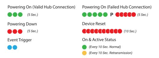
**NOTE:** If the Sensor is out of range or the Hub unit was not turned on, the status LED on the Sensor will start rapidly blinking red after power up. Make sure the Hub unit was turned ON first or try relocating the Sensor/Hub combination so they are closer to each other. Power cycle or reset Sensor to retry Hub unit connectivity validation. (For further troubleshooting refer to hardware user manual)
