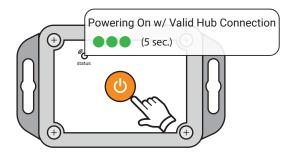
1.) Press and release the power/function button; the status light blinks green.
