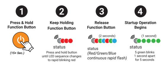
**NOTE:** During holding the function button the status light sequence will pass though the sensitivity menu in which the status light will start blinking green/red. Continue to hold past this until the status light is only rapidly blinking red.
