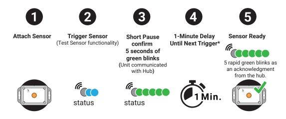
(\*One minute trigger is only for the 1st through 5th trigger. The 6th trigger and after is a one hour backoff. The timer resets if the unit's heartbeat goes out, power cycled or a reed trigger will set it back)
