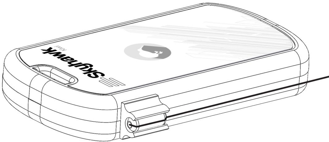
**Step 6:** Tie other end of filament line to the object being monitored such as a door or trap; making sure that when tripped, the line will pull easily from the magnet mount on the Kiwi.
